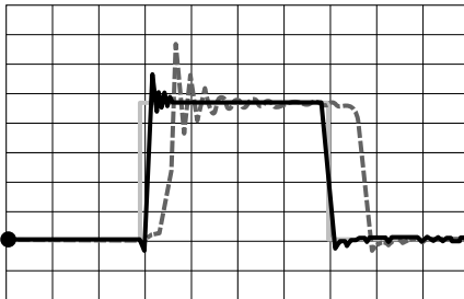
— GaN --- MOS FET — Ideal Switching Waveform
